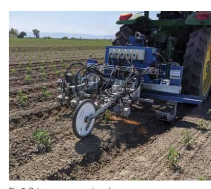
Fig. 2. Robovator, automated weeder
