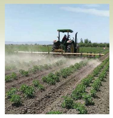
Fig. 3. Finger weeder, mechanical weeder
