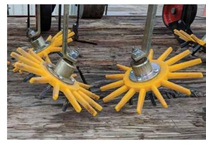
Fig. 1. Close-up of the finger weeder mechanism
