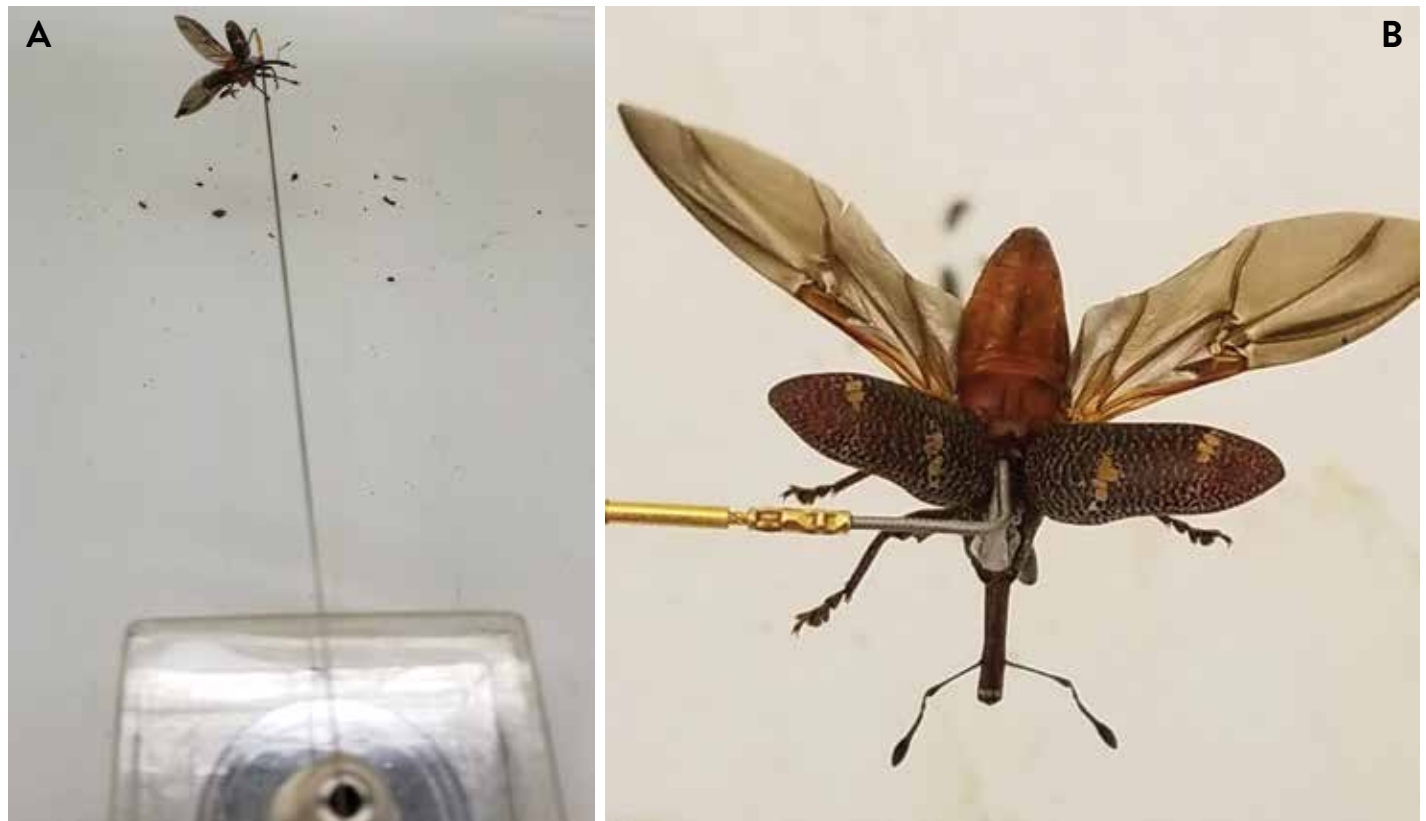
Fig. 6. (A) Heilipus lauri attached to a flight mill arm which spins in circles when the weevil flies. (B) A close-up of the harness that is glued to the weevil's thorax. The harness is attached to the flight mill arm. Photos: Mark Hoddle, UC Riverside
