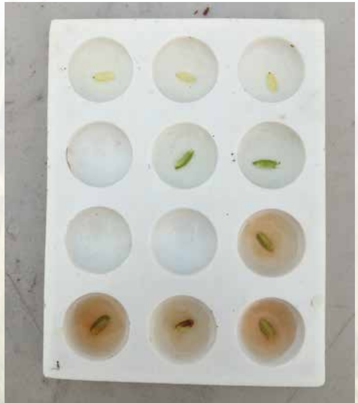
FIG. 6. Potassium hydroxide (KOH) test shows pericarp of weedy rice stained red, while cultivated varieties (control) remain white. Photo: Luis Espino, UCCE
