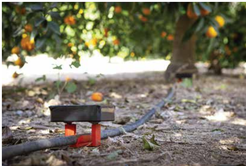
FIG. 5. IR sensor clamped onto an irrigation line in a commercial citrus orchard. Photo: Mike Lewis
